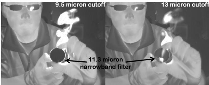
**Figure 2.** Images of Center for Quantum Devices graduate student Edward Huang holding a lighter and a narrow-band filter centered at  $11.3\mu\text{m}$ . The flame can be seen when imaged with the bandpass detectors sensitive up to  $13\mu\text{m}$  (right), but not in the ones with shorter-detection wavelengths up to  $9.5\mu\text{m}$  (left).
