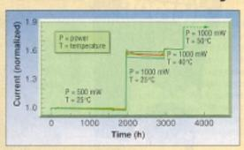
Ongoing tests suggest both rugged operation and long life for indium gallium arsenide phosphide (InGaAsP) based aluminumfree diode lasers fabricated by researchers at Northwestern University (Evanston, IL). Elimination of aluminum removes an easily oxidized specie that spreads performance-degrading defects through the structure by forming light-absorbing dark lines or spots (see Laser Focus World, Aug. 1994, p. 26).
