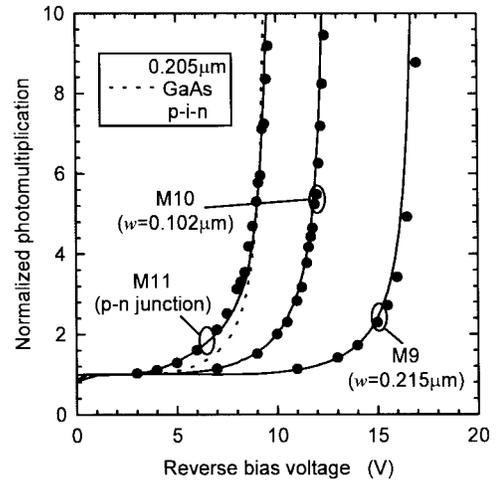
Fig. 3.  $M_h$  ( $\approx M_e$ ) for M11 ( $p$ - $n$  junction), M10 ( $w = 0.102 \mu\text{m}$ ), and M9 ( $w = 0.215 \mu\text{m}$ )  $\text{Ga}_{0.52}\text{In}_{0.48}\text{P}$   $p$ - $i$ - $n$  devices (—) from left to right.  $M_e$  for the  $0.205 \mu\text{m}$  GaAs  $p$ - $i$ - $n$  device (— — —) is also shown. Symbols represent results from the Monte Carlo model (see text).
