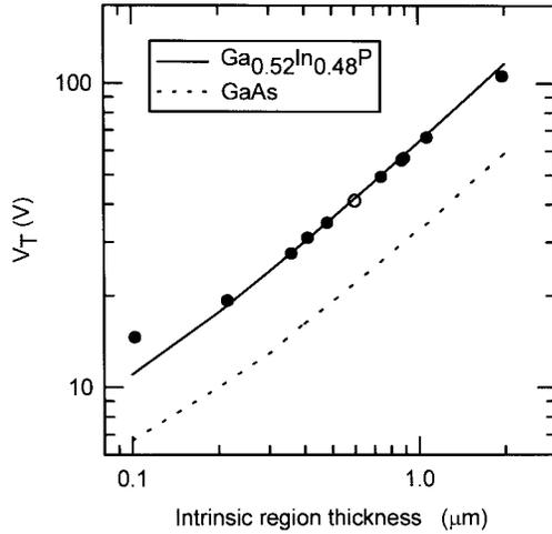
Fig. 4. Calculated breakdown voltage for Ga<sub>0.52</sub>In<sub>0.48</sub>P (—) from present parametrised form of  $\alpha$  and  $\beta$ , and for GaAs [17], [18] (- - -) plotted for ideal p-i-n devices as a function of the *i*-region thickness. Measured values for Ga<sub>0.52</sub>In<sub>0.48</sub>P from present data (●) and from [1] (○) are also shown.
