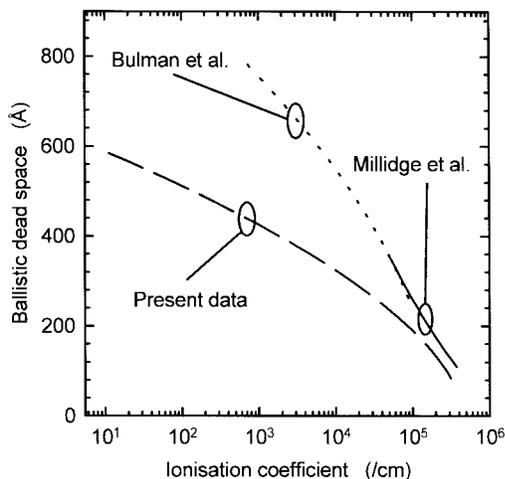
Fig. 6. Ballistic dead space plotted as a function of the ionization coefficient for GaAs from [17] (—), [18] (---), and  $\text{Ga}_{0.52}\text{In}_{0.48}\text{P}$  (---).
