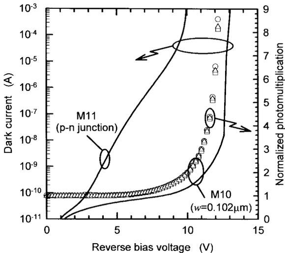
Fig. 2. Normalized photomultiplication values for M10 ( $w = 0.102 \mu\text{m}$   $p$ - $i$ - $n$ ) using top injection of 442 nm ( $\circ$ ), 542 nm ( $\square$ ), and 633 nm ( $\Delta$ ) excitation wavelengths. In addition, dark currents (lines) for M10 and M11 ( $p$ - $n$  junction) are shown.
