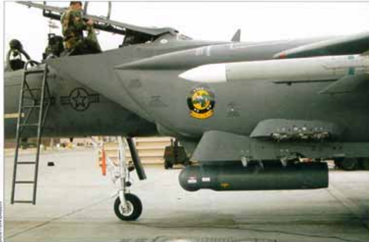
The Litening II pod, shown mounted beneath an F-15 fighter, contains infrared and CCD detectors to identify targets and a laser designator for precise delivery of munitions.
