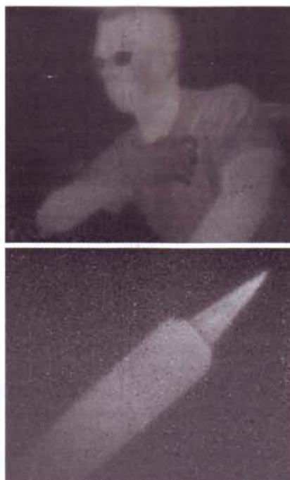
FIGURE 2. A thermal image of the human body (top) was produced by a QDIP focal-plane array operating at 130 K; a soldering iron (bottom) was imaged at 200 K.
