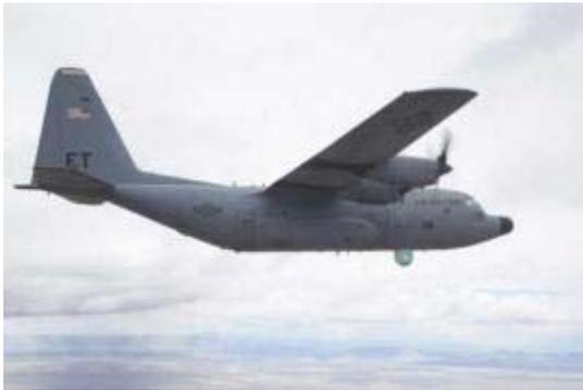
The Advanced Tactical Laser will use a rotating ball turret to fire its laser weapon at ground targets.
