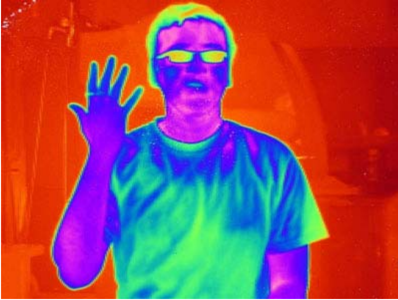
Image of CQD graduate student Paritosh Manurkar taken with the world's first LWIR FPA based on Type-II superlattices.
