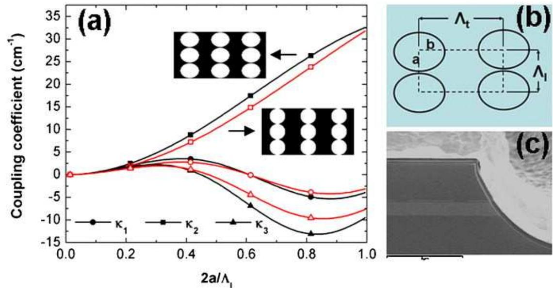
(a)  $\kappa_1$ ,  $\kappa_2$ , and  $\kappa_3$  coupling coefficients of rectangular PhC lattice with an aspect ratio of 2 with elliptical and circular features. (b) Depiction of the rectangular lattice dimensions with elliptical holes. (c) The cross section view of a cleaved facet and buried gratings on the finalized device.
