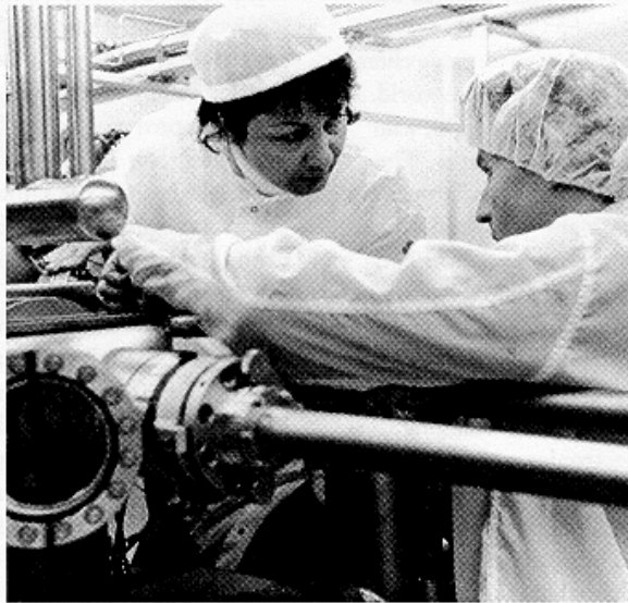
Razeghi and Philippe Bove, a visiting postdoctoral scientist, discuss the molecular beam epitaxy reactor, in which laser wafers are grown.
