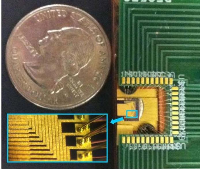
**Figure 1.** Fully packaged distributed feedback quantum cascade laser array compared with a US quarter. This device can operate in continuous-wave mode with a wavelength coverage of 4.5–4.7 $\mu$ m at room temperature.
