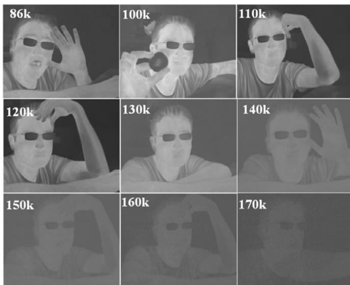
**Figure 3.** Mid-wavelength IR images of a student captured with a T2SL focal plane array at a range of temperatures.
